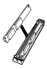
6. Push the SIMM into the socket until it is seated firmly in the slot. Then tilt it upright, as shown below, guiding the hole at each end of the SIMM over the retaining post at each end of the SIMM socket. If it does not go in smoothly, do not force it; pull it all the way out and try again.
